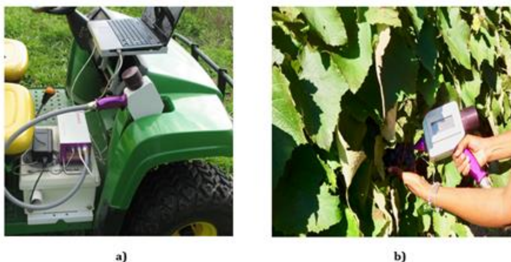
Figure 1 Demonstration of spectra taking in the field, (a) detail of the integration of equipment to Gator. (b) Collection of the spectrum using the NIR spectrophotometer
